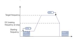
Dual-frequency braking. Generate large braking torque, greatly shorten stopping time and apply to the cases with a high requirement on braking time.
